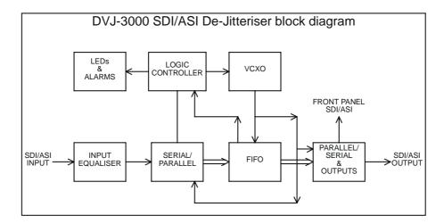
The DVJ-3000 is designed to reduce the jitter in 270 Mb/s SDI or ASI signals.
