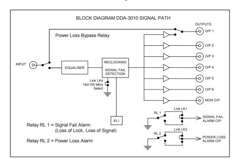
The IRT DDA-3010 is a single input, six out 140/155 Mb/s data distribution amplifier whose input and outputs comply with ITU Rec. G.703.
