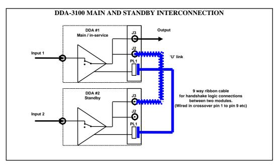
It is important to note that in this mode only one output (J 2 / J 3) of the DDA-3100 is switched and outputs J 4 and J 5 on either DDA-3100 cannot be relied upon in this mode and should therefore normally not be used.
