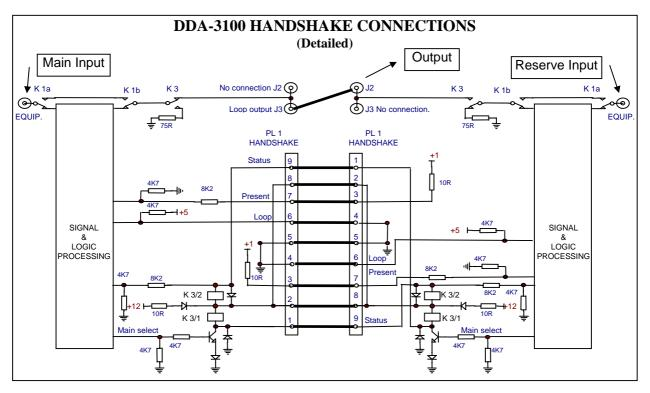
The handshake kit GMW-3100 provides the necessary connections for operating two DDA-3100's for paired operation as shown in the diagram. The kit provides both a 1.6/5.6 'U' link and a data cable to cross connect two adjacent modules in a standard 3 RU frame.
