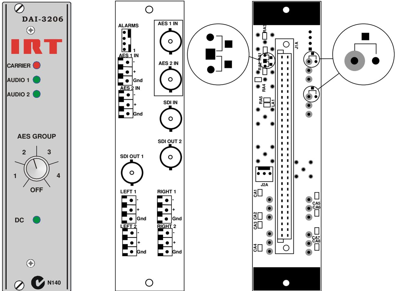
Underside of rear assembly with areas marked with a ■ indicating where to connect together to convert to a 75 Ohm unbalanced AES input.
