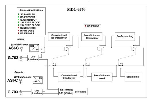
The MDC-3570 is part of a family of data transcoders for converting between the commonly used MPEG2 Transport Stream formats in the broadcast industry for video distribution.
