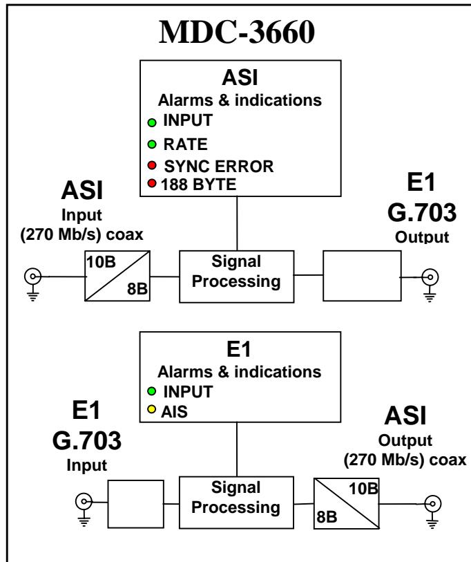
The MDC-3660 takes a 2048 kb/s G.703 (E1) signal and packs it into an RS encoded DVB compliant, 204 byte, ASI transport stream. This allows it to pass through ASI style of circuits such IRT's ASI Mux/DeMux and fibre modules.
