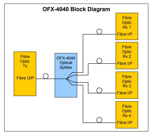
The OFX-4040 is an optical splitter suitable for use with IRT's complete range of optical fibre transmitters comprising of HD, SD, ASI, L-Band or analogue signals.
