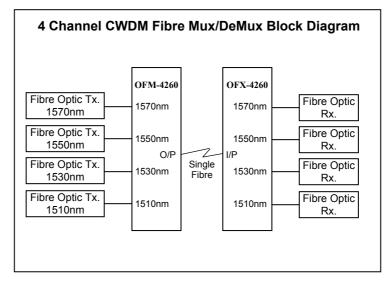
The OFM-4260 and OFX-4260 form a coarse wave division optical wavelength division multiplexer / demultiplexer (CWDM) pair for combining and separating up to four optical signals of 1510nm, 1530nm, 1550nm and 1570nm wavelengths for uni-directional transmission on the one fibre.
