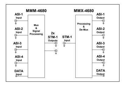
The MMM-4680 (Iss. 2) and MMX-4680 (Iss. 2) are part of a family of data transcoders for converting between the commonly used MPEG2 Transport Stream formats for video distribution in the broadcast industry.
