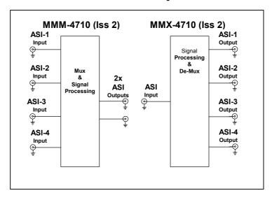
The MMM-4710 (Iss. 2) and MMX-4710 (Iss. 2) are part of a family of data transcoders for converting between the commonly used MPEG2 Transport Stream formats for video distribution in the broadcast industry.
