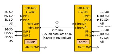
NOTE: \* Fitted with APD detector. 3-18dB when fitted with PIN detector.
