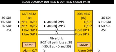
NOTE: \* Fitted with APD detector. 3-18dB when fitted with PIN detector.
