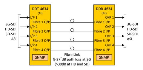
NOTE: \* Fitted with APD detector. 3-18dB when fitted with PIN detector.
