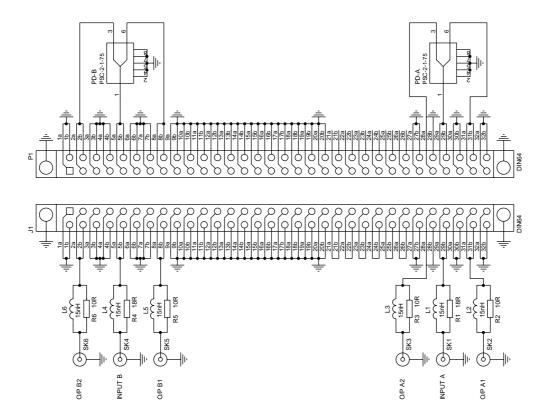
Changes from DDF-3100 module Ouput 1 from PD-A moved from pins 27a,b to pin 28a. Pins 27a,b grounded. Pins 21a,b to 26a,b removed from the DIN64 plug on the module.
