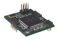
The SMU-4000 is a Simple Network Management Protocol (SNMP) plug-in interface option for IRT 4000 series modules when used in IRT's SNMP capable frames.
