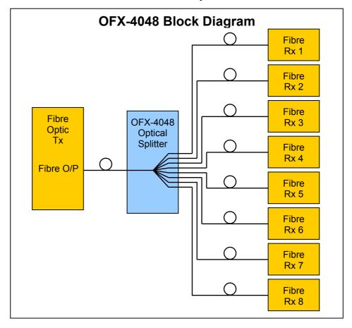
The OFX-4048 is an optical splitter suitable for use with IRT's complete range of optical fibre transmitters comprising of HD, SD, ASI, L-Band or analogue signals.
