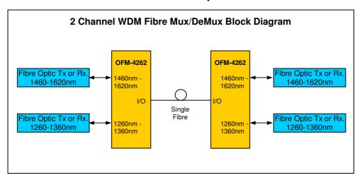
The OFM-4262 is wave division optical wavelength division multiplexer / demultiplexer (WDM) for combining and separating two optical signals of 1260-1360nm (typically 1310nm) and 1460-1620nm (typically 1550nm) wavelengths for either uni-directional or bi-directional transmission on the one fibre.
