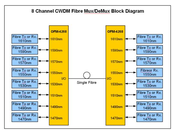
The OFM-4268 is coarse wave division optical wavelength division multiplexer / demultiplexer (CWDM) for combining and separating up to eight optical signals of 1470nm, 1490nm, 1510nm, 1530nm, 1550nm, 1570nm, 1590nm and 1610nm wavelengths for either uni-directional or bi-directional transmission on the one fibre.
