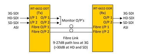
The IRT-6632-DDT and IRT-6632-DDR are dual transmit and receive modules designed principally for use as two independent serial data fibre optic transmission links for 3G-SDI, HD-SDI or SD-SDI applications conforming to SMPTE standards 424M, 292M and 259M-C using 9/125  $\mu$ m single mode fibre. This enables the use of space saving fibre optic cable for reliable transmission of digital video signals over lengths greater than can be achieved with coaxial cable.
