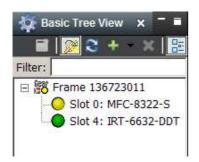
On the left the basic tree view shows the frame. With the tree structure expanded a list of cards within the frame is shown. In this example, slot position 4 is IRT-6632-DDT. When selected, all sections and tabs to the right of the basic tree view now relate to the card in slot position 4. The name of the card, in this case IRT-6632-DDT, can be set under its Configuration TAB setting.
