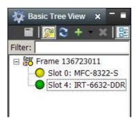
On the left the basic tree view shows the frame. With the tree structure expanded a list of cards within the frame is shown. In this example, slot position 4 is IRT-6632-DDR. When selected, all sections and tabs to the right of the basic tree view now relate to the card in slot position 4. The name of the card, in this case IRT-6632-DDR, can be set under its Configuration TAB setting.
